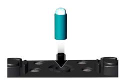
⇒ The touch valve must be approx. 9.7 mm above the suction cup connection plate.
