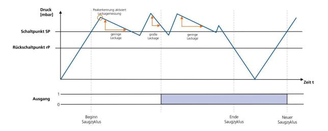
Another application for condition monitoring mode occurs if the regulation threshold of the vacuum system is never achieved and the vacuum generator permanently drains. In this case, if the end vacuum is 20 mbar lower than the start vacuum, the switching point will also be activated.
