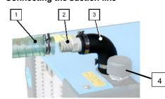
Connect the machine-side line for the gases/vapours (suction line) to be transported to the connection piece of the suction nozzle (pos. 037).
