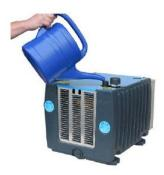
Pour an additional 1.5I operating liquid into the suction nozzle (pos. A) of the system, so that operating liquid enters the interior of the integrated unit.
